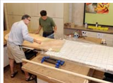
Mark Chidister (left) and Randy Fiscus slide a tabletop quadrant into the vacuum bag before boosting the pressure inside it during gluing.
