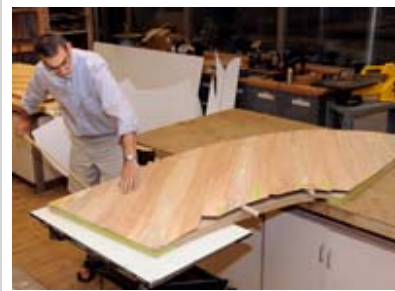
Mark Chidister used a series of dowels to center the maple veneer layer on the tabletop section during gluing.
