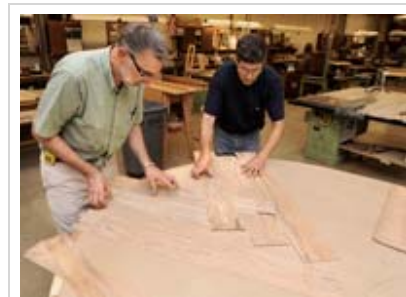
Mark Chidister (left) and Randy Fiscus begin the task of laying out the veneer strips.
